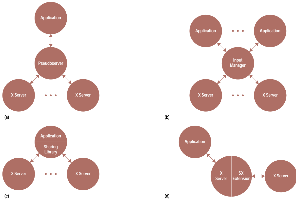
Fig. 5. Different application sharing architectures. (a) Centralized pseudoserver architecture. (b) Replicated architecture. (c) Sharing-library architecture. (d) Integrated architecture.
