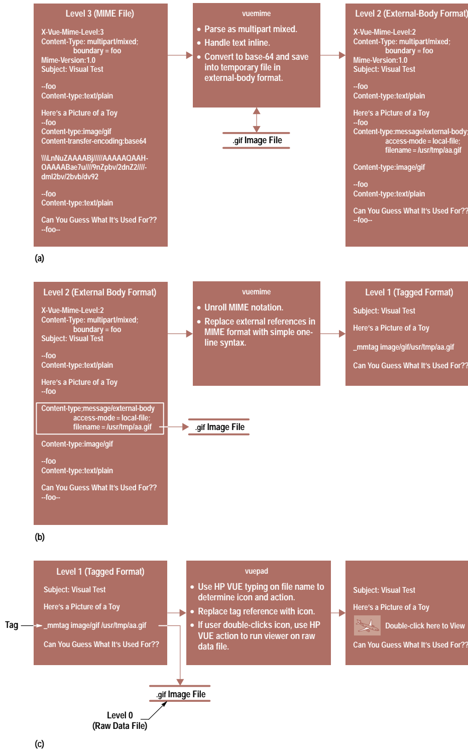
Fig. 4. Processing an incoming message. (a) Level-3 file format and the actions of vuemime to move from a MIME format to a level-2 file format. (b) Level-2 file format and the actions performed by vuemime to transform the data to a level-1 representation. (c) Level-1 file format representation and the actions taken by vuepad to display textual and nontextual parts of the message.
